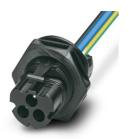
Device connector rear mounting, Range of articles: PRC 35, housing material: PPE, color: black, number of positions: 3, max. conductor cross section: 4 mm², rated voltage: 690 V AC, rated current: 32 A, Connection method: Crimp connection, Contact connection type: Pin, This item is also available with other cable lengths. For your specific requirements, please contact your local PHOENIX CONTACT subsidiary.
